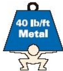
A 60" spiral metal duct weighs 40 lbs./ft. (18 gauge, single wall)
